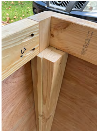
Overbuilt the framing with 2x4s and pocket screws to hide the joints.
