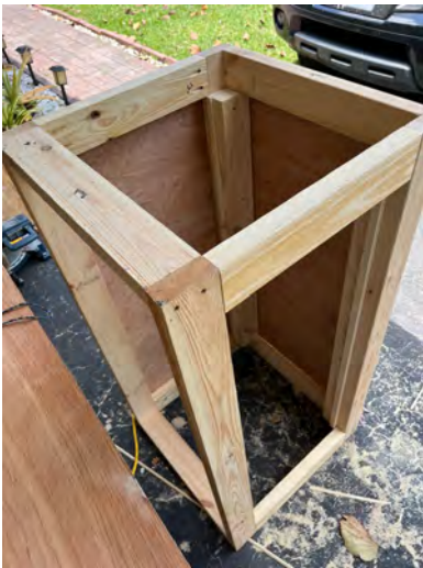
Overbuilt the framing with 2x4s and pocket screws to hide the joints.
