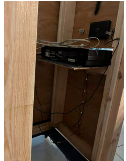
The LED install using hot glue and gaff tape.
